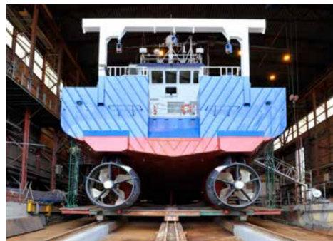
Figure 3.9: Gunnerus fitted with two PM-AZ thrusters [56]
