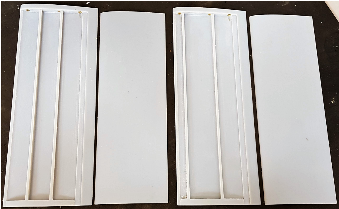
Figure 4.13: The two foils that was printed with Stratasys 3D printer at SINTEF Ocean. They were printed in two parts and glued together as on Figure 4.14
