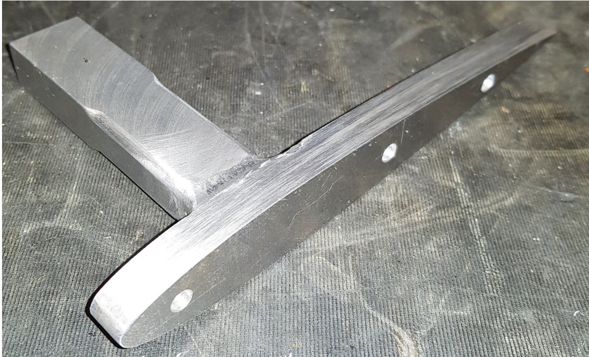
Figure 4.12: Picture of the shaft that was designed and was attached on the top of the printed foils. The cutting was conducted at SINTEF.
