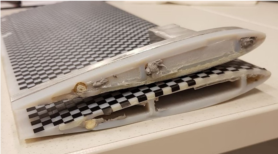
Figure 5.3: Picture of the foil that broke during testing at f_m = 0.95 Hz. It broke at the glued part. It is possible that the glue was not strong enough to sustain the bending moment close to the fixed end
