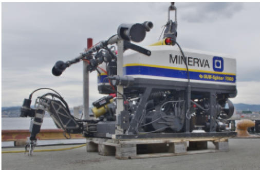
(c) Class III ROV, Minerva
