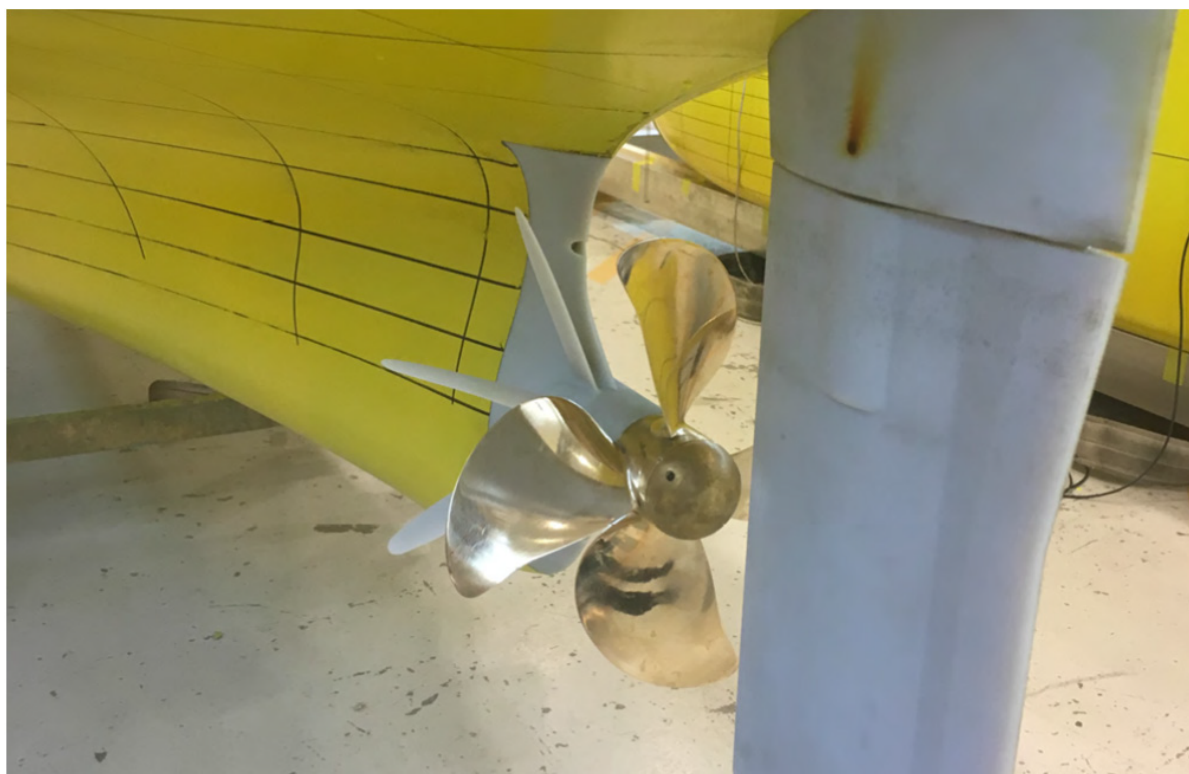
Figure 1.3: Propulsion test setup with designed PSS (Krasilnikov et al., 2019).
