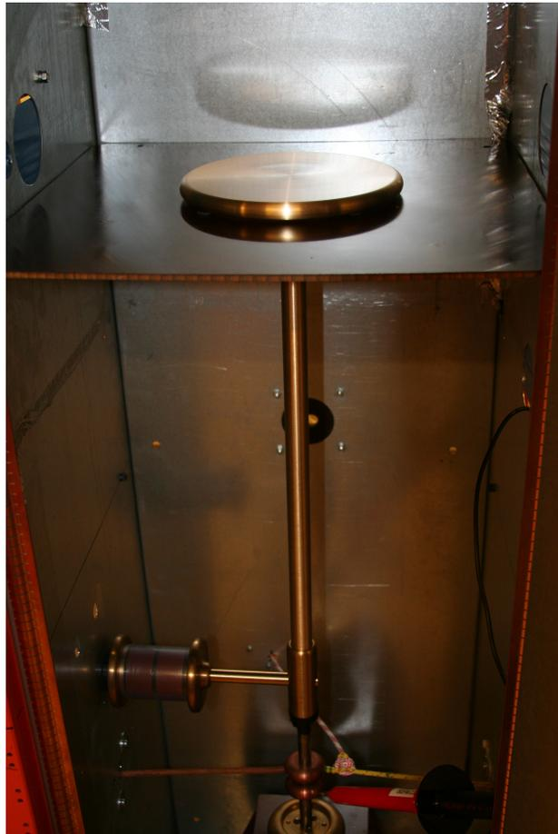
Figure 5.9: Top electrode connected to the transformer
