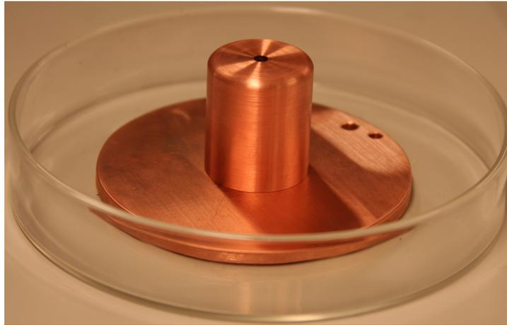
Figure 5.6: Test object for fast rise time repetitive pulses with drilled holes for banana plugs
