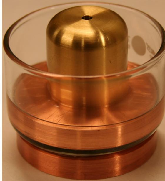
Figure 5.7: Test object for AC testing
