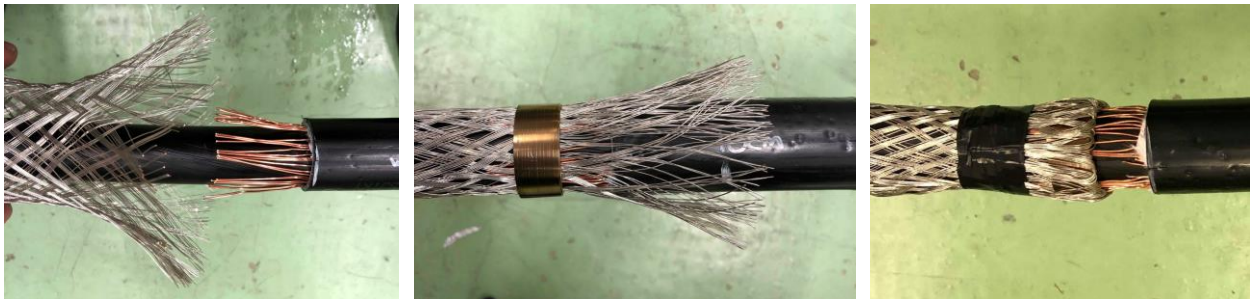
Picture 2 – Installation of test object
