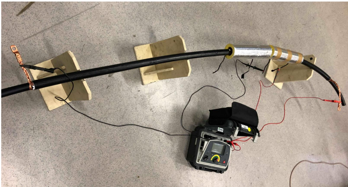
Picture 7 – Resistance measurement from the short circuit test
