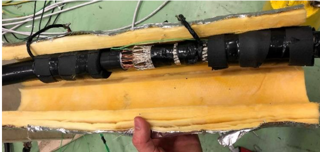
a) Test object isolated with 13 mm black Armaflex pipe insulation
