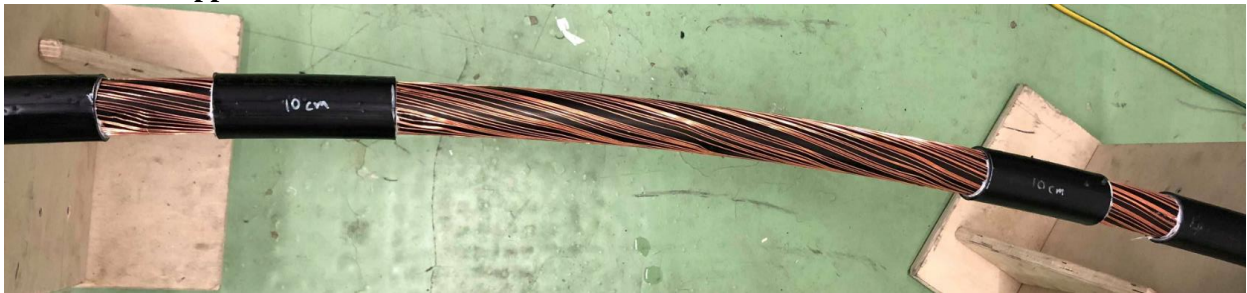
Picture 1 – Stripped cable sheath
