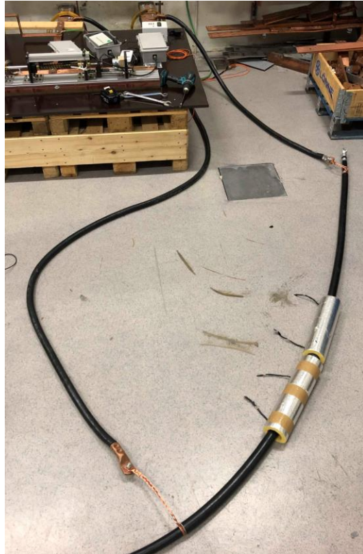
Picture 6 – Short circuit test setup
