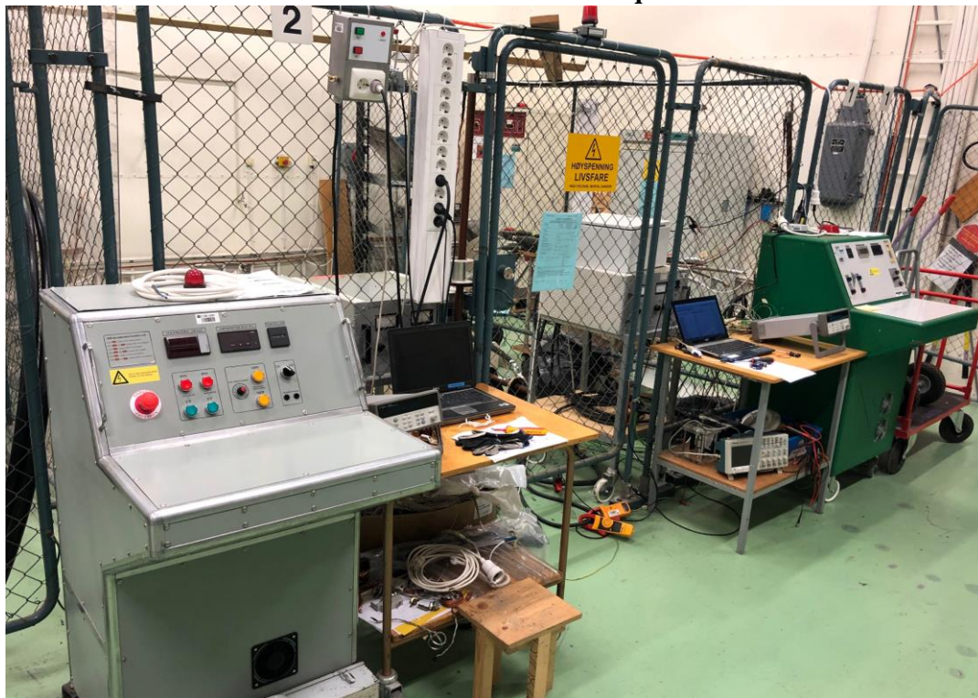
Picture 5 – Control units and data acquisition tools
