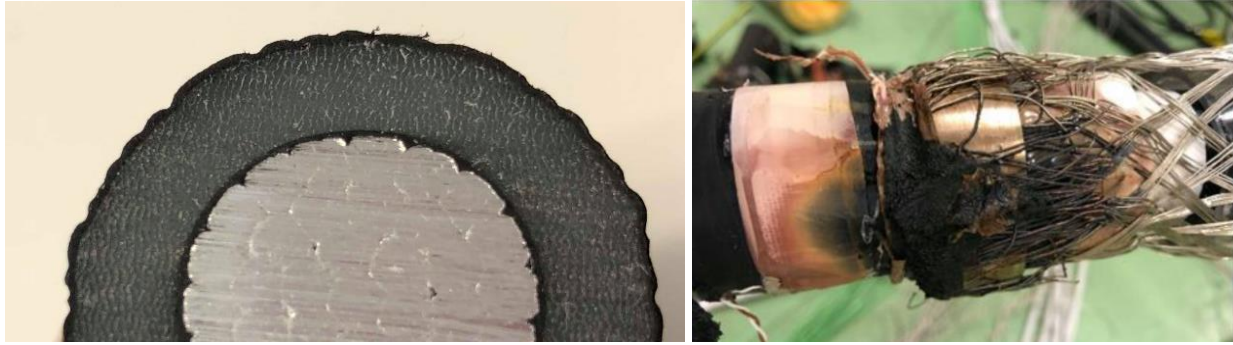
Figure 1.1. Deformations in XLPE insulation and hotspot caused by an incorrectly installed force spring. [3]
