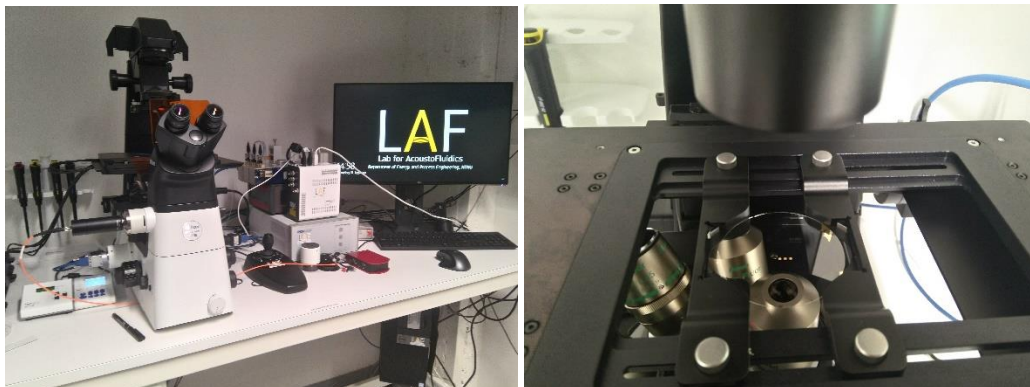
Figure 24 – Left hand image, overview of the facility setup. Right hand image, close view of the setup, light source on top, nanoplasmonic sensor and magnification on the bottom.
