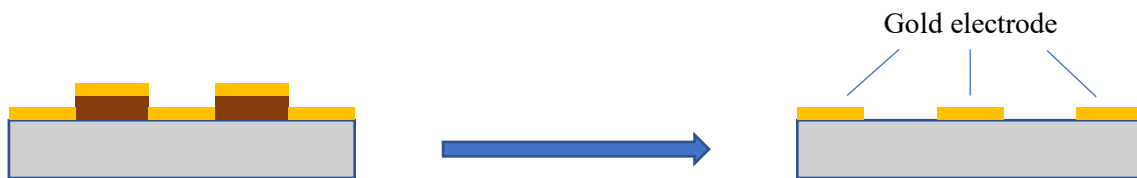
Figure 59: Lift-off representation process.
