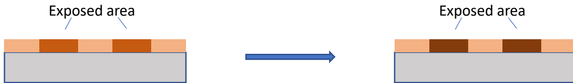
Figure 11: Post-exposure baking representation.
