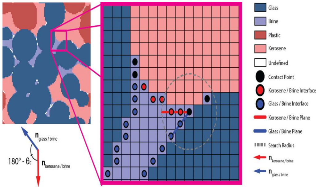
Figure 18: Klise et al. (2016) method to estimate contact angles in kerosene-brine-glass system [20].
