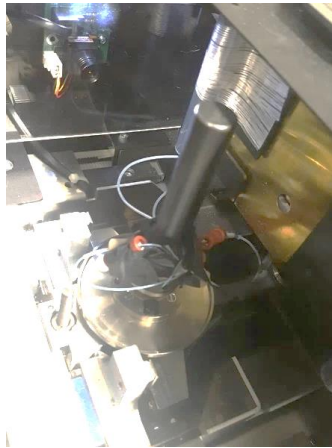
Figure 41: The core-holder and tubes fixed on the scanner stage
