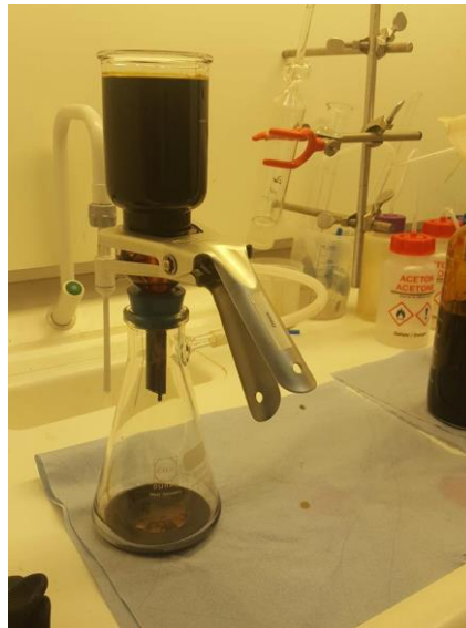
Figure 61: Setup for filtering the crude oil under vacuum
