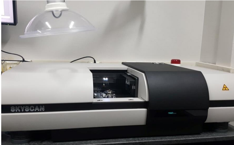
Figure 40: SkyScan 1172 micro-CT scanner used for the experiments of this study
