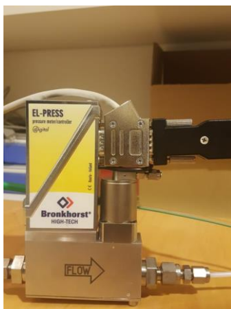
Figure 42: A high accuracy back-pressure regulator used in the setup of this study
