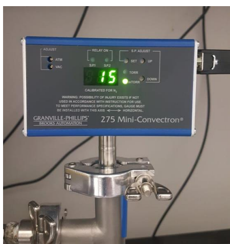
Figure 44: Vacuum gauge showing 15 millitorr pressure in the setup system
