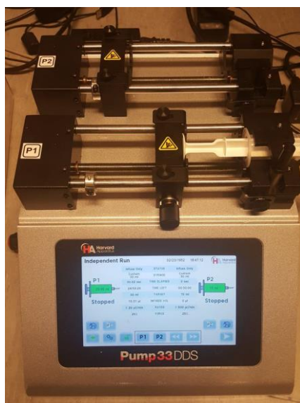
Figure 43: Harvard Apparatus pump 33 DDS (dual drive system) used in the setup of this study
