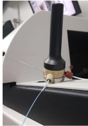
Figure 39: Core-holder manufactured by Reservoir Study Systems (RSS), Norway
