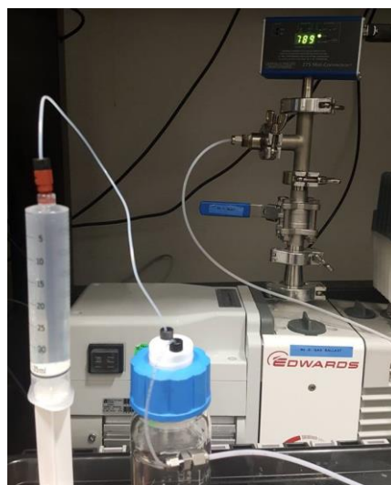
Figure 63: Demonstration of connecting the syringe to the degassing system to remove the air bubbles
