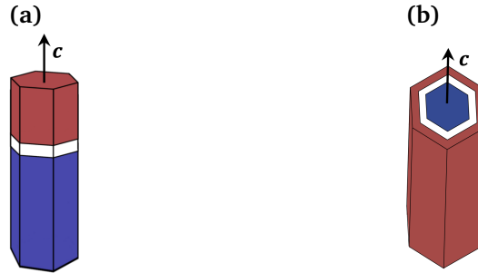
Figure 2.1: Illustration of hexagonal NW with (a) an axial heterostructure, where different layers are grown in the c -direction and (b) a radial heterostructure, where layers are grown perpendicular to the c -axis. It is also possible to grow structures composed of a mixture of the two.
