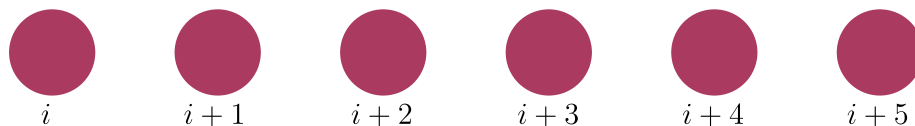
Figure 2.1: A schematic overview of the lattice structure in a ferromagnet. Here, i is an integer, and the burgundy circles are lattice sites, for which the distance between them is a .
