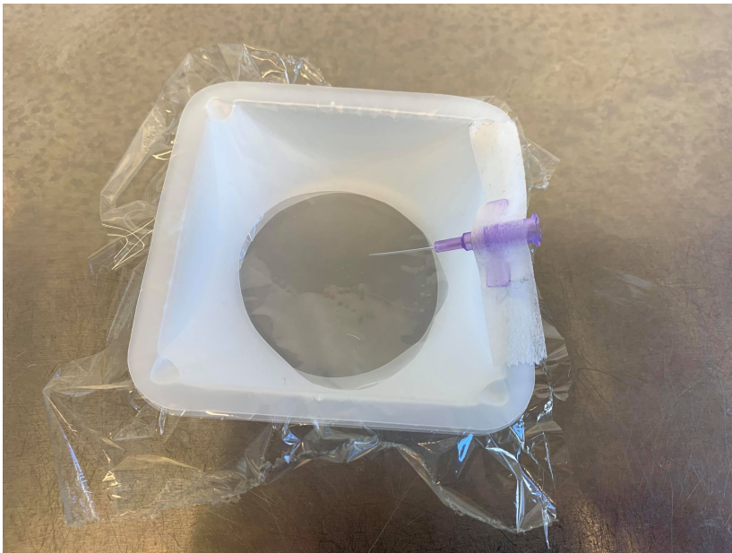
Figure 3.8: The catheter was taped to the wall of the weighing boat during the experiments.
