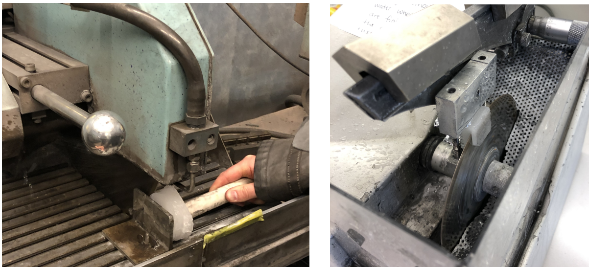
Figure 3.6 Cutting of fused silica sample. Left: coarse cutting, Right: fine cutting
