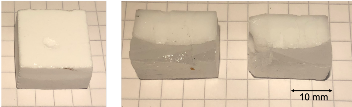
Figure 4.5 A trial fused silica sample with a thick, complete layer of cristobalite after a validating viscosity measurement. Left: indented surface. Right: cross-section
