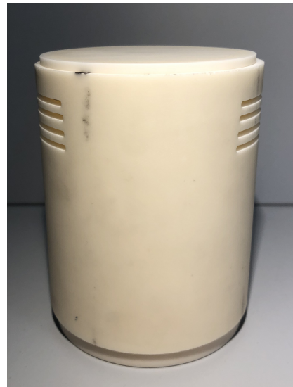
Figure 3.1 Crucible for fused silica production
