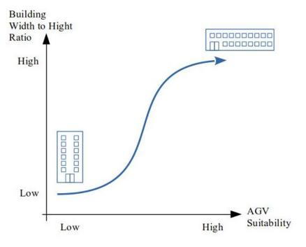
Figure 12: AGV suitability diagram
