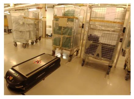
Figure 7: An AGV about to pick up a hamper
