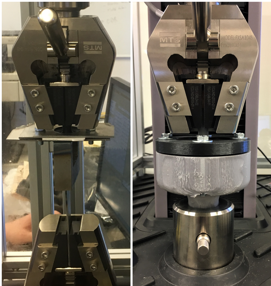
Figure 3.21: Image of the metal jig (left) and the 3D-printed (right) jig attached to the machine.
