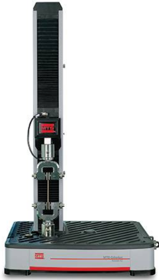
Figure 3.20: MTS Criterion Model 42 (left) [40] and welded test jig attached to the machine (right)
