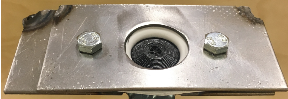
Figure 4.11: Point of failure on the transition between the pinhead and the narrowest part of the pin
