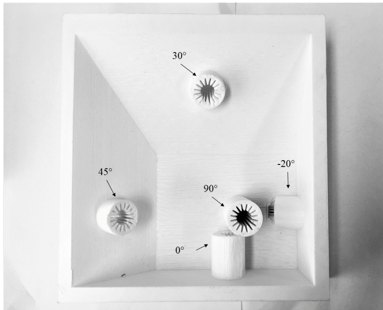
Figure 5.3: Picture of the placement of vent holes on the inside of the angled mold. Notice that all the vent holes, except 0^\circ and -20^\circ , are pointed downwards (or out if the image) when the mold is placed right side up.
