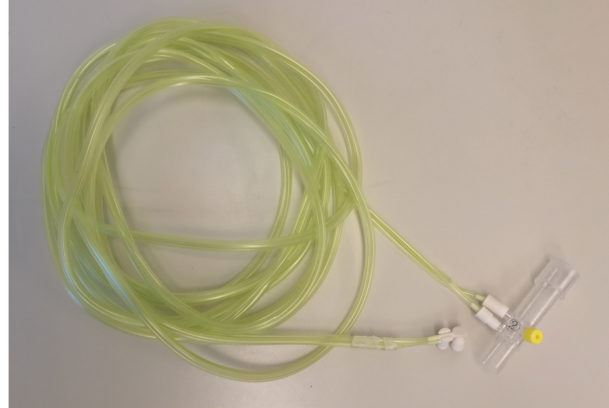
Figure 4.8: The flowmeter and spirometer tube setup
