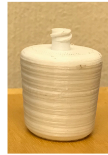
(c) The cap showing visible grooves, indicating poor printing quality
