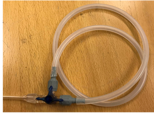
(b) The female to female luer lock prototype, shown with the two female connectors connected to the male ports on a three-way connector
