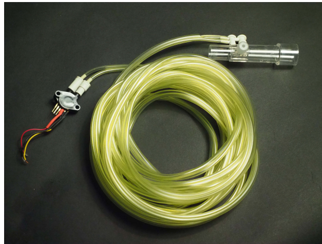
Figure 5.6: The flowmeter test setup, showing the MPX5010DP ports and flowmeter ports connected to the spirometer tube
