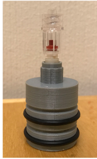
(a) The finished cap with o-rings and a one-way valve
