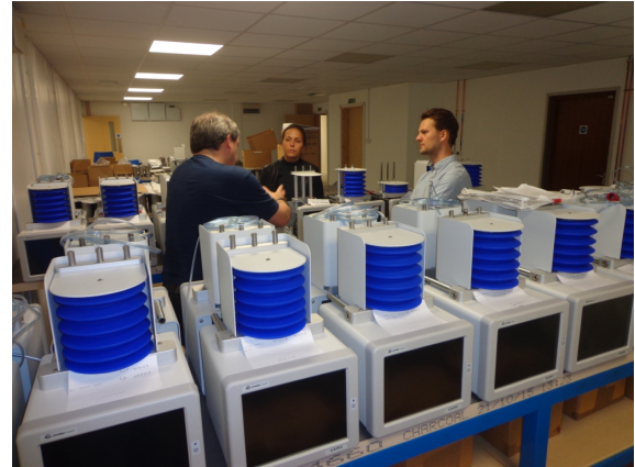
(b) Automatic ventilators used in the UAM. Photograph taken at the OES factory
