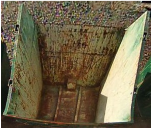
(c) Very rusty container.
