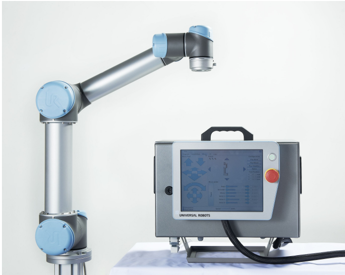
Figure 5.1: Overview of the Universal Robots UR5 Robot system. It consists of three components: The robot manipulator, the controller box centred on the table, and the teach pendant attached to the controller box. Picture in courtesy of [79]
