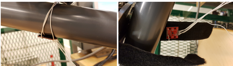
(a) Accelerometer placement when measuring without manipulator attached (b) Accelerometer placement when measuring with manipulator attached
