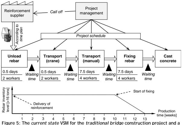
schematically drawn diagram of the actual superstructure rebar inventory level.
