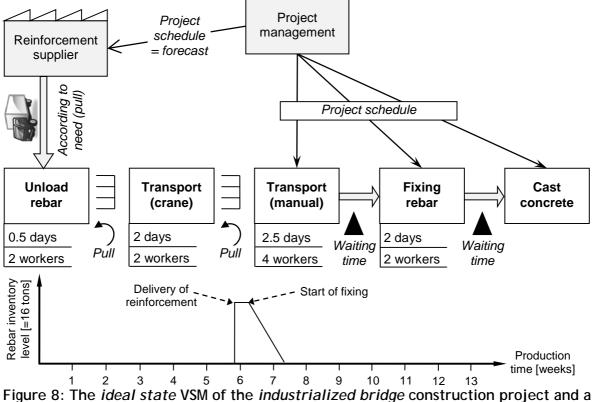
Figure 8: The *ideal state* VSM of the *industrialized bridge* construction project and a schematically drawn diagram of the actual superstructure rebar inventory level.
