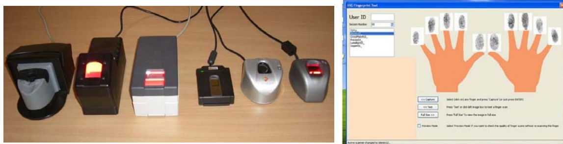
Figure 2. Left: fingerprint sensors used to collect data for GUC100 (from left to right): TST BiRD 3, L-1 DFR 2100, Cross Match L SCAN 100, Precise 250 MC, Lumidigm V 100 and Sagem MorphoSmart; Right: interface of the data collection program.
