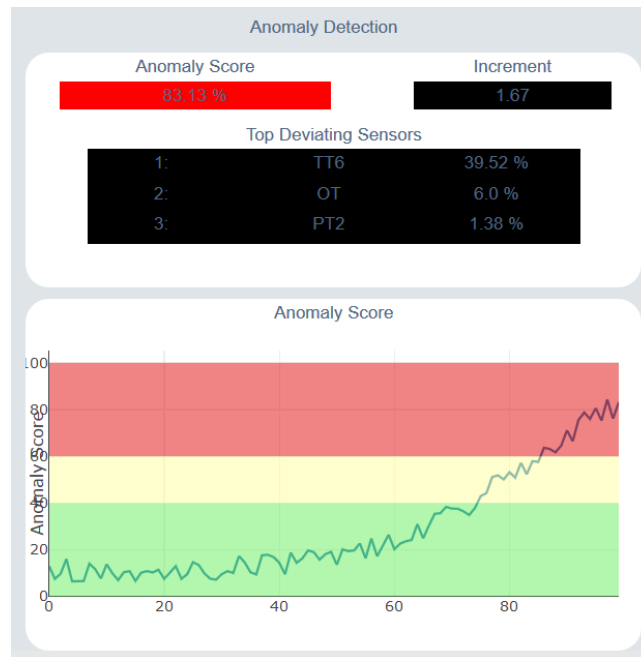
Figure 3: Anomaly detection in demo PHM-application
