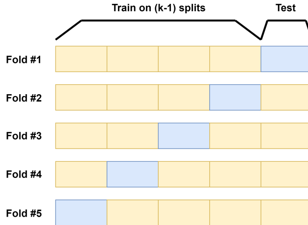
Figure 4.1: K-fold cross validation process with 5 folds
