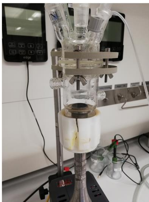
b. Broken cap during a Fricke dosimetry test
