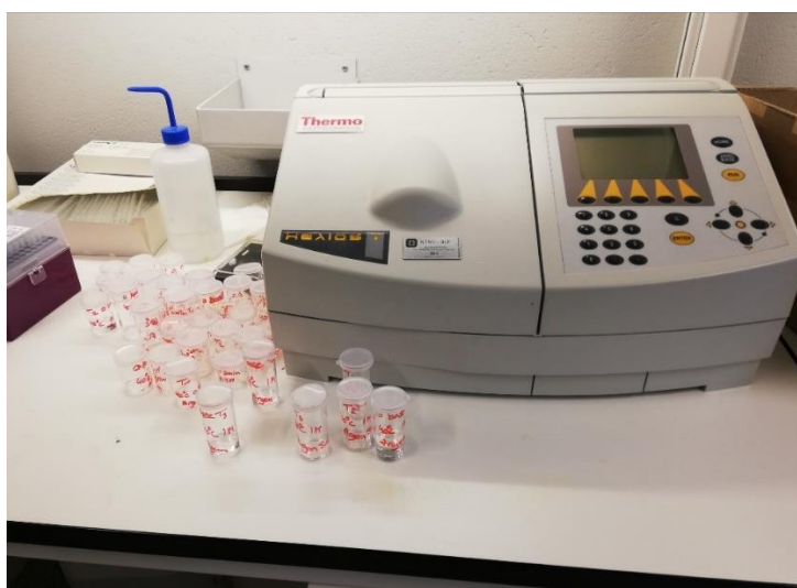
Figure 10: Testing of samples with Helios Gamma spectrophotometer
