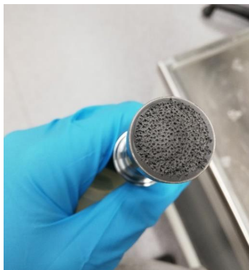
Figure 3: Erosion effects observed in an ultrasonic horn made with titanium
