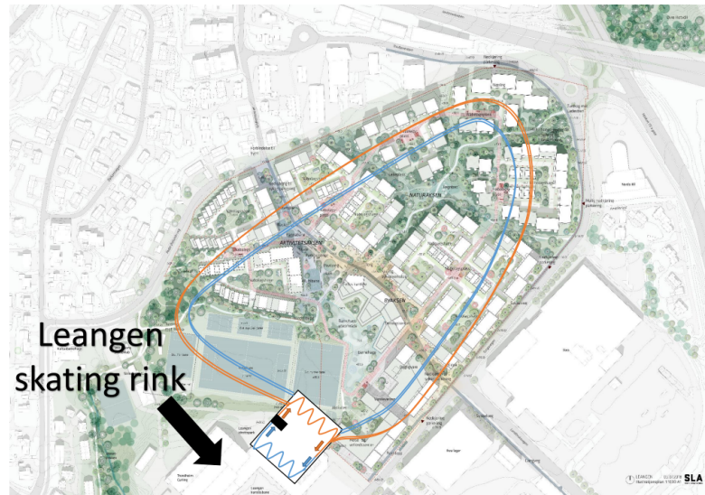
Figure 29: Illustration of low-temperature network at Leangen
