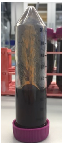
Figure 4.9: Heat-treated RRM after centrifugation. Orange material scattered on the tube surface is assumed to be a solid lipid fraction.
