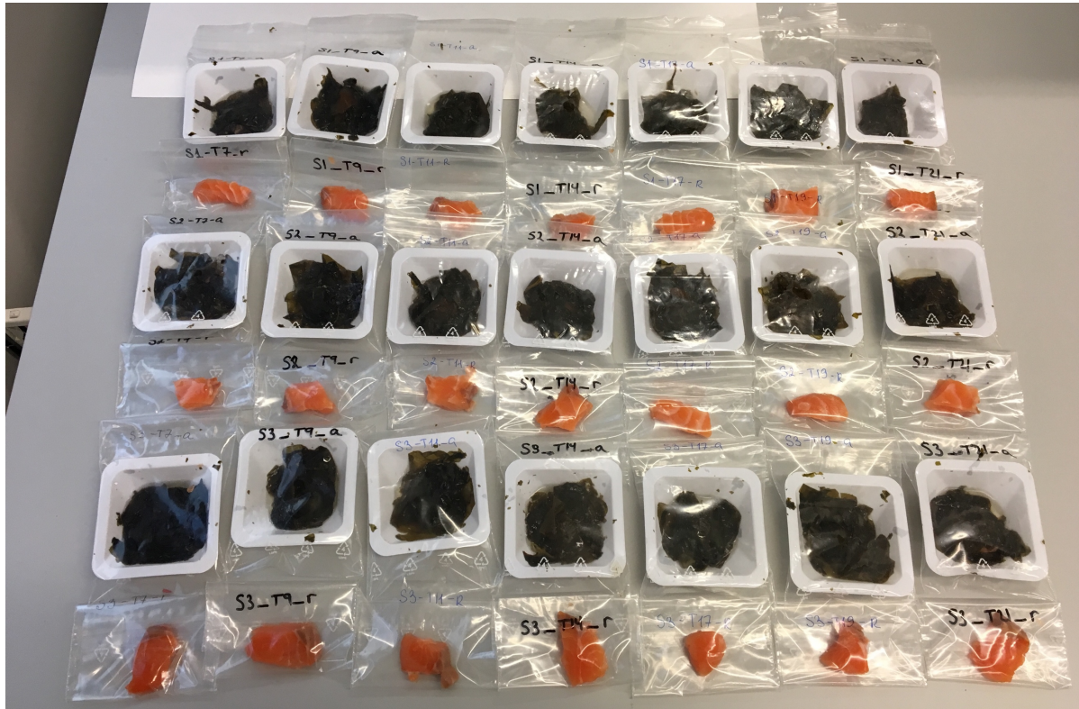
Figure 2.3. Overview of premium quality salmon (PQS) and sugar kelp samples prepared for storage. After storage, polar metabolites were extracted by trichloroacetic acid (TCA) and analyzed with 1D ^1\text{H} NMR spectroscopy.
