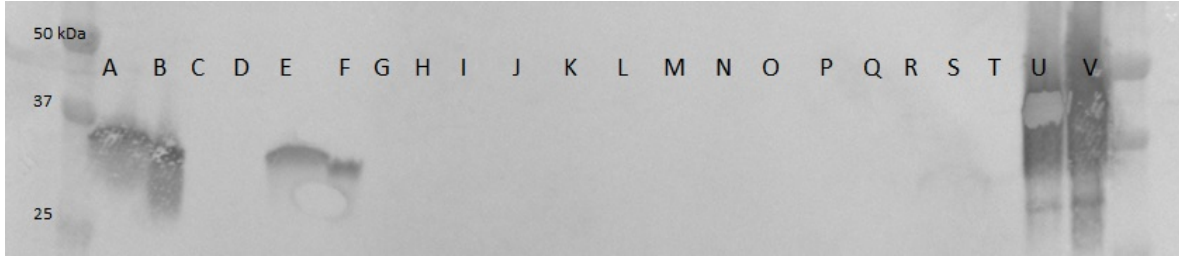
Figure 3.7: Expression of \sigma^{32} from pMSM69.4 construct over 4 time points; 1.5, 3, 5 and 20 hours post induction. After harvesting, lysates were separated into soluble (S) and insoluble (I) fractions and 10 \mu L of undiluted lysate was loaded onto the gel. Lane A: 1.5 hr S/In; lane B: 1.5 hr I/In; lane C: 1.5 hr S/Un; lane D: 1.5 hr I/Un; lane E: 3 hr S/In; lane F: 3 hr I/In; lane G: 3 hr S/Un; lane H: 3 hr I/Un; lane I: 5 hr S/In; lane J: 5 hr I/In; lane K: 5 hr S/Un; lane L: 5 hr I/Un; lane M: 20 hr S/In; lane N: 20 hr I/In; lane O: 20 hr S/Un; lane P: 20 hr I/Un; lane Q: 20 hr pVB-1A0B1-mCherry S/In; lane R: 20 hr pVB-1A0B1-mCherry I/In; lane S: 20 hr pVB-1A0B1-mCherry S/Un; lane T: 20 hr pVB-1A0B1-mCherry I/Un; lane U: \sigma^{32} standard 50 ng; lane V: \sigma^{32} standard 100 ng. Ladder used is Precision Plus Protein Standards Dual Color from Bio-Rad (kDa). Induced (In), Uninduced (Un).
