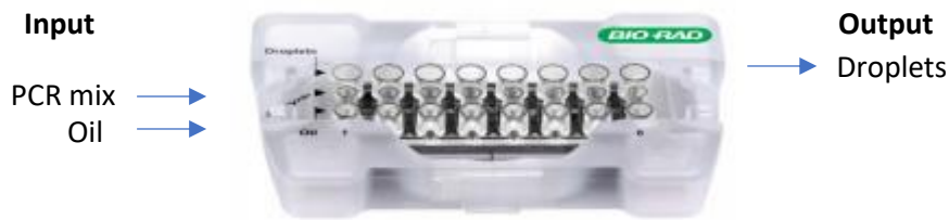
Figure 21. ddPCR cartridge for droplet generation. The cartridge with 20uL of PCR mix and 70uL of oil goes into the droplet generator to generate the droplets.
