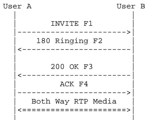
In this scenario, User A completes a call to User B directly. The call from A to B is marked with a resource priority indication.
