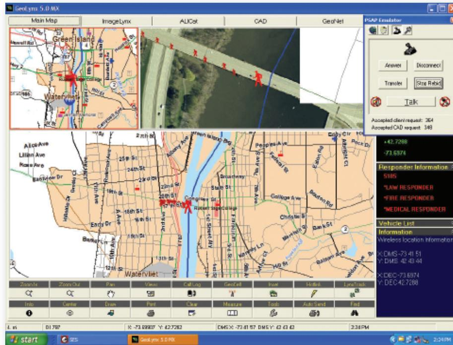
A shared emergency management screen showing an entire moving incident. Thanks to the “multi directional” capability of IP, information was shared over the IP infrastructure from 2 PSAPs and displayed, complete, on the CARM emergency management display.
