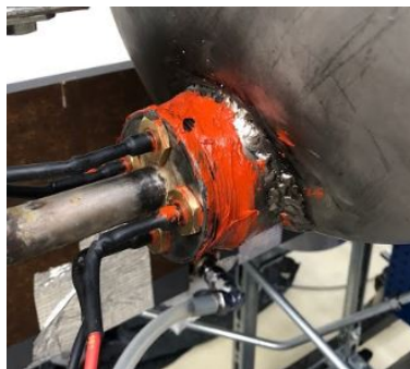
Figure 56: The plug with the heating elements and the bimetallic spring sealed into the storage tank
