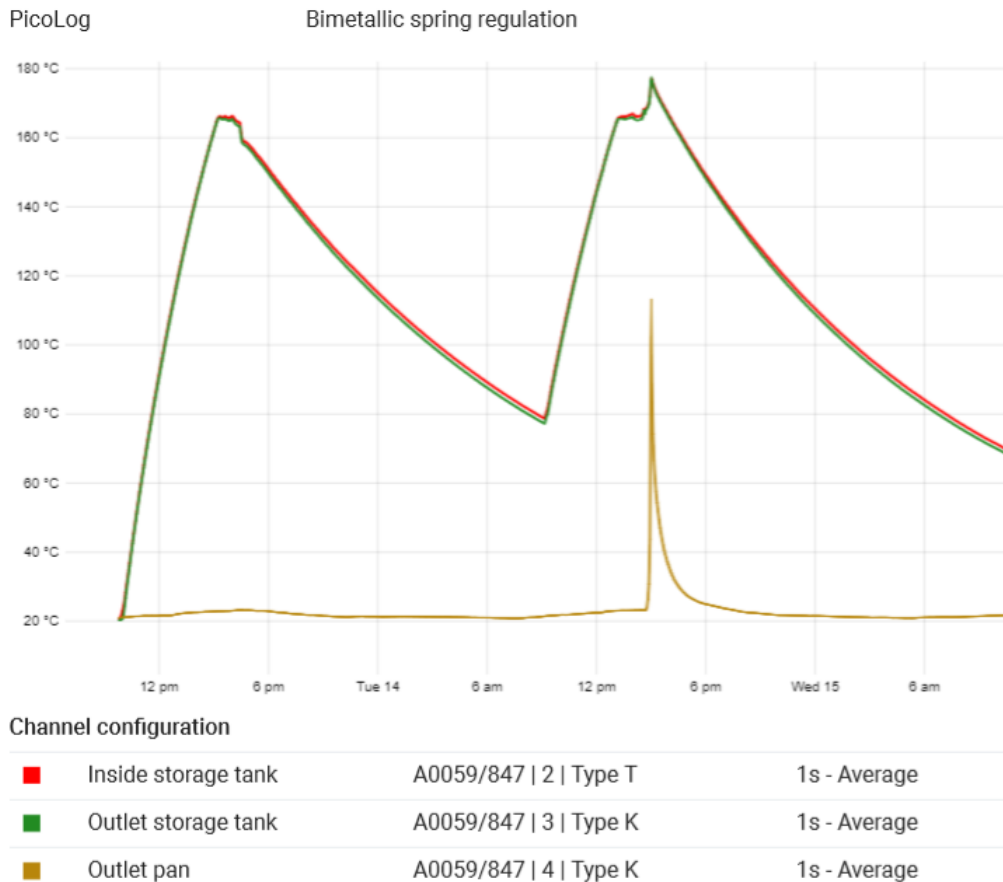
Figure 64: Test of bimetallic spring over 2 days
