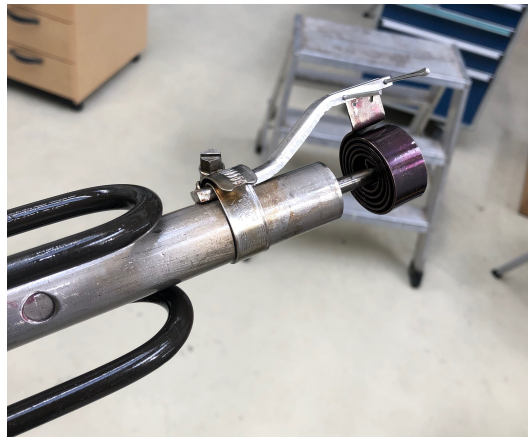
Figure 51: Bimetallic spring mounted on slider and pipe
