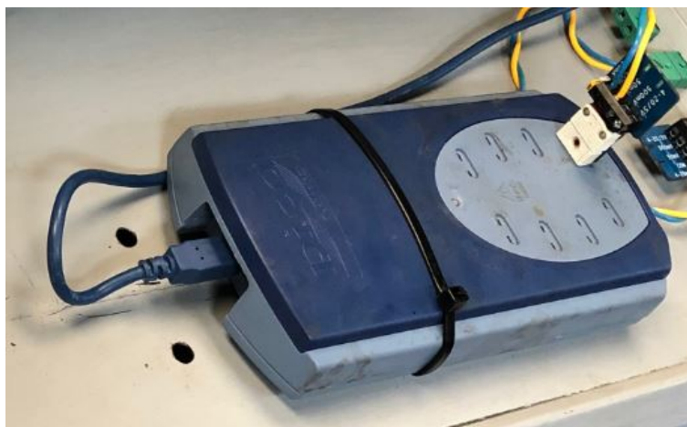
Figure 27: The terminal board connected to the PicoLog system
