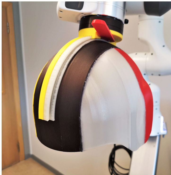
Figure 3.15: The 3D printed helmet with slider and magnetic connection mounted to the robot
