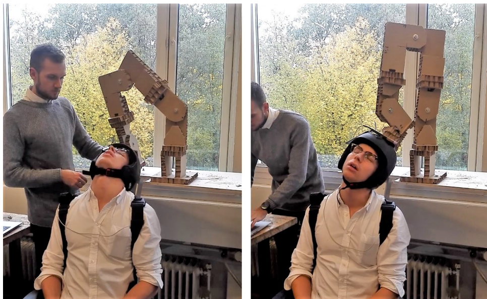
Figure 3.5: Two of the extreme positions of the head tested with the model attached in position 1
