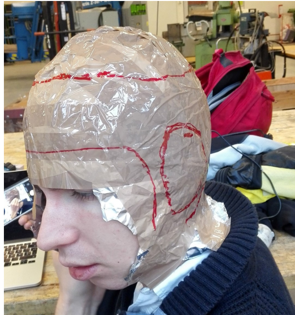
Figure 3.8: Template with markings for the boundary of the inflatable element
