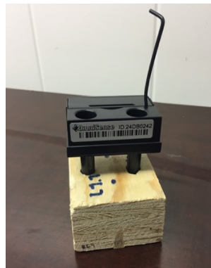
Figure 1: Omnisense sensor placed in an LVL sample, with the electrodes perpendicular to the grain direction
