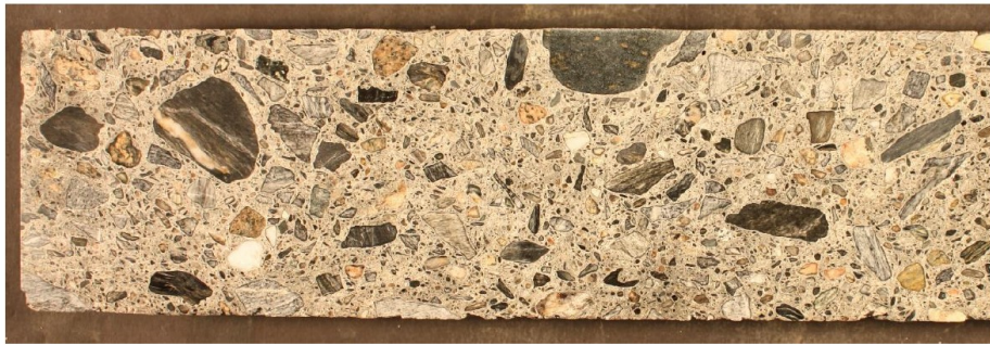
Figure A7 : Polished section of the Dam Tyn 4, 470 - 770 mm specimen.
