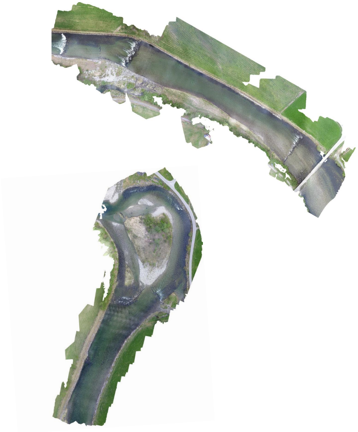
Figure H 5: Ortophotomosaic of two parts of Lærdaselva. The picture on the top corresponds to Øye and it has a total error of 5cm. The figure on the bottom corresponds to Ofta and it has a total error of 7cm
