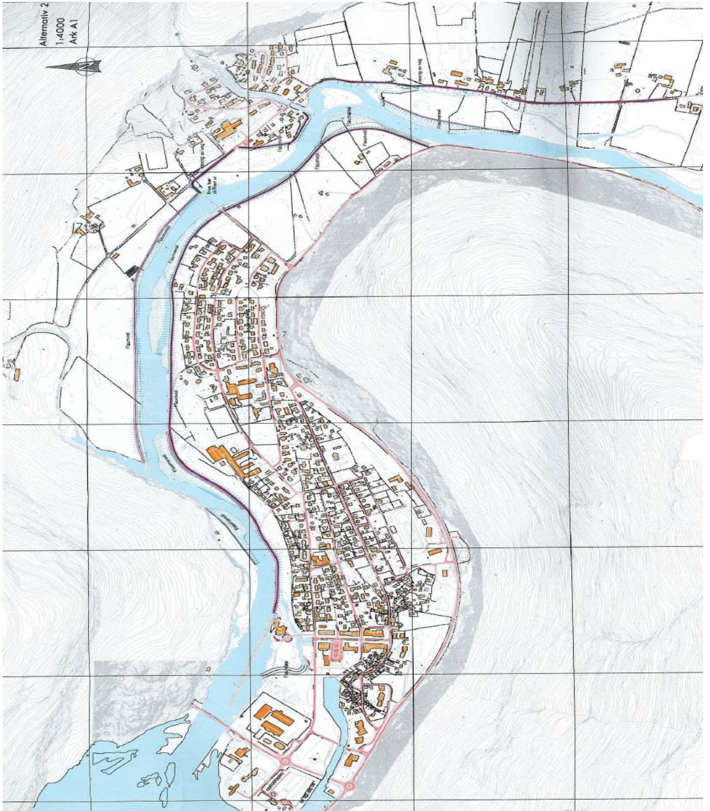
Figure A.2: Alternative 2 of the flood protection plans for Lærdal developed by NVE
