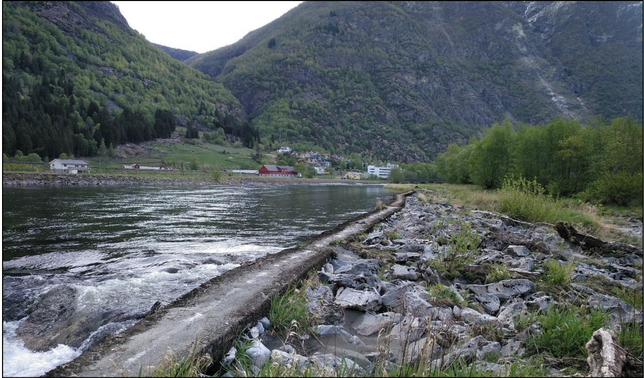
Figure H.3: Area classified as Gravel 2. It is in this location where the highest differences between the GPS and the green LiDAR values were obtained
