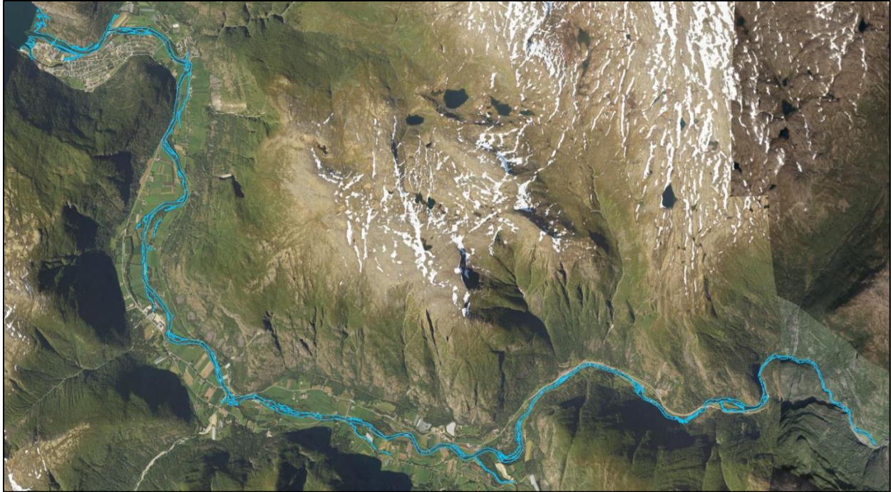
Figure 8: Water edge line (blue line) obtained from an aerial photograph taken the day of the flight when the underwater bathymetry data was collected (29.05.2018).
