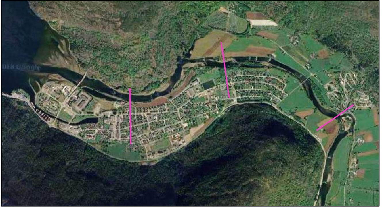
Figure G 3: Profile lines selected to check the WSE and the effect of the wall in some cross sections
