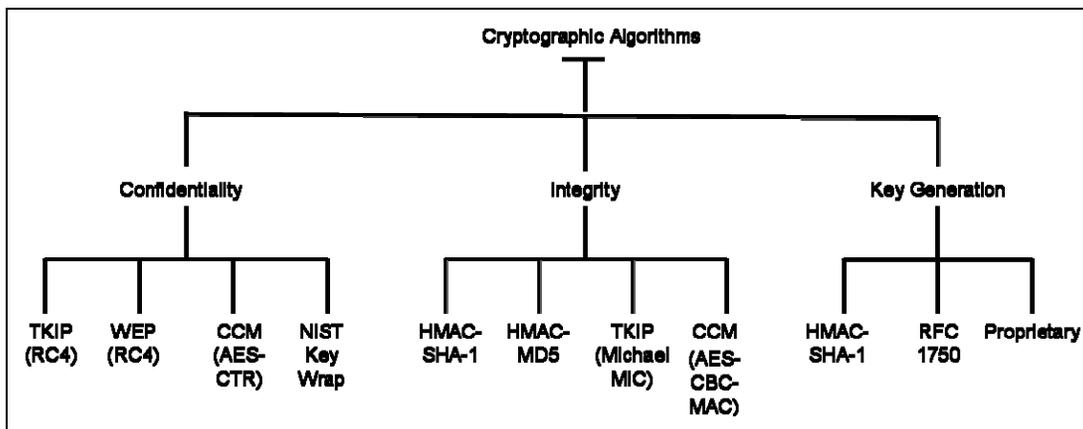
Figure 4-3. Cryptographic Algorithms Used in IEEE 802.11<sup>26</sup>
