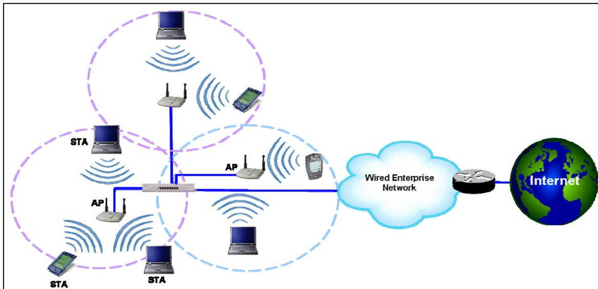
Figure 2-3. Extended Service Set in an Enterprise
