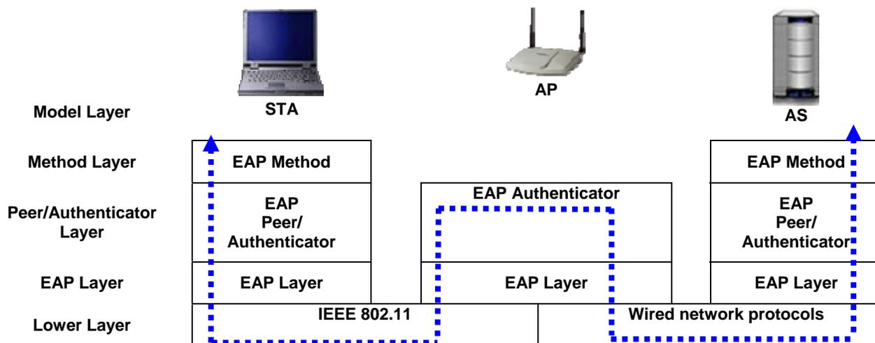
**Figure 6-5. EAP Traffic Flow in IEEE 802.11 RSN**
