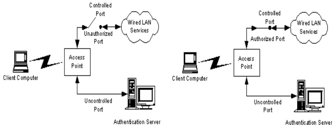
This diagram shows both the uncontrolled port used for authentication requests and the controlled port in its pre-authentication setting (left) and post-authentication setting (right.) As you can see, when a supplicant is successfully authenticated, the controlled port is considered authorized and communication through the logical port is allowed.
