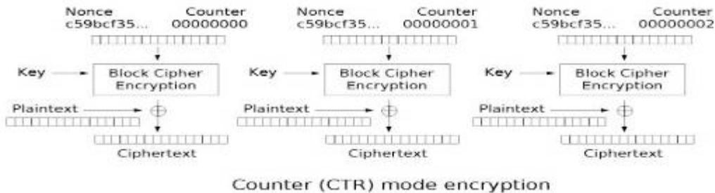
As you can notice, there is a random nonce that is added to the counter and then is added to the AES temporal key to encrypt the plaintext. The nonce is created by CCMP's implementation of what WEP and TKIP call their Initialization vector or IV. CCMP calls the value the PN Value. The PN value is 48 bits in length and
