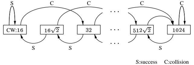
Fig. 2. Backoff mechanism of EIED:  $CW_{\min} = 16$ ,  $CW_{\max} = 1024$ ,  $r_I = 2$ ,  $r_D = \sqrt{2}$ .
