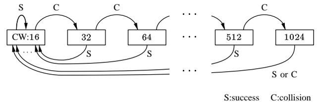
Fig. 1. Backoff mechanism of BEB:  $CW_{\min} = 16$ ,  $CW_{\max} = 1024$ ,  $m = 7$ .
