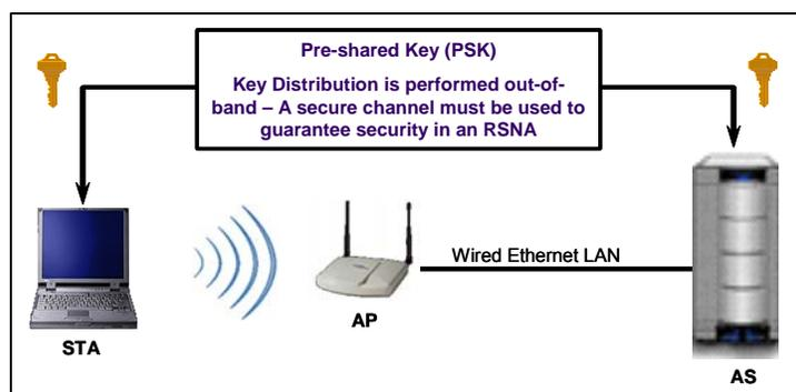
Figure 4-5. Out-of-Band Key Distribution for the PSK
