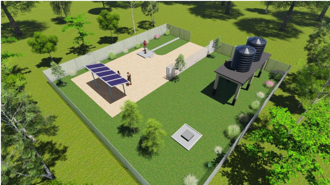
Figure 8.1: Schematic drawing of multiple use of water services (MuS), installed in NCA's TCP (WAYD Designs obtained from private email correspondence with NCA staff, 8 th of May 2019).
