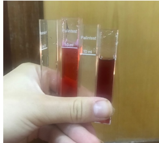
Figure 4.3: Samples from two different locations, where the saturation of red indicates the concentration of fluoride in the water sample.
