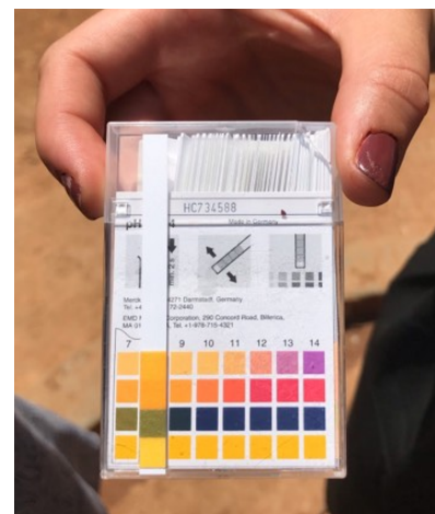
Figure 4.2: pH testing in field showing a pH value of approximately 7.
