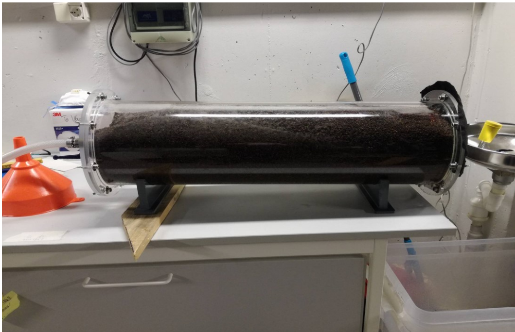
Figure A3.1. Lab column test for estimations of hydraulic conductivity in both unfrozen and frozen aggregate conditions.
