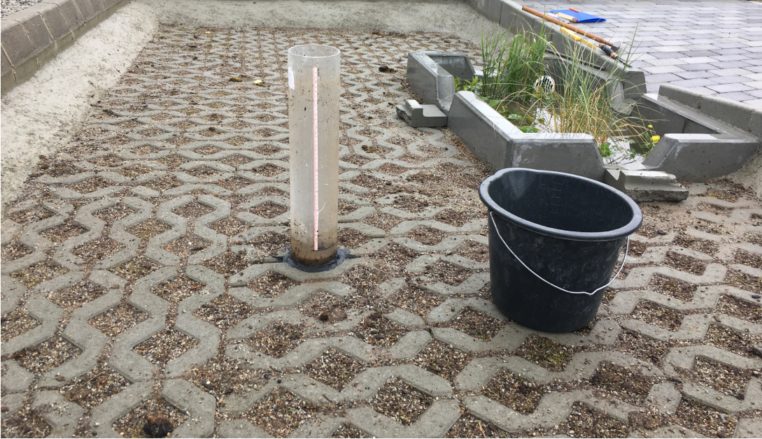
Figure A3: The MPD test, indicating the measurement location and the way it was placed on the surface using silicon. The post-experiment ponding water in Alma was stayed at weir level.
