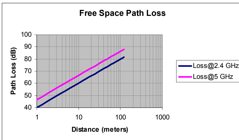
Figure 1: Free space path loss at 2.4 GHz and 5 GHz
