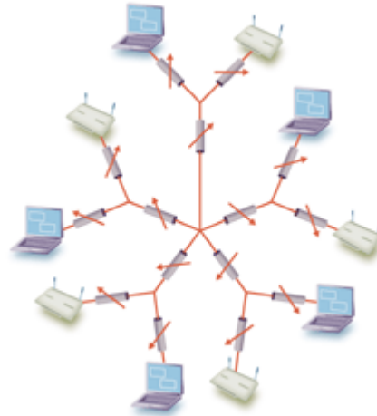
Figure 2. RF cables connect to the 50-V antenna ports of the devices-under-test with antennas removed. Programmable RF attenuator settings emulate physical distances between devices.
