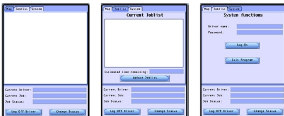
Figure 6.4: Field application GUI. Map view (left), joblist view (centre) and logon view (right).
