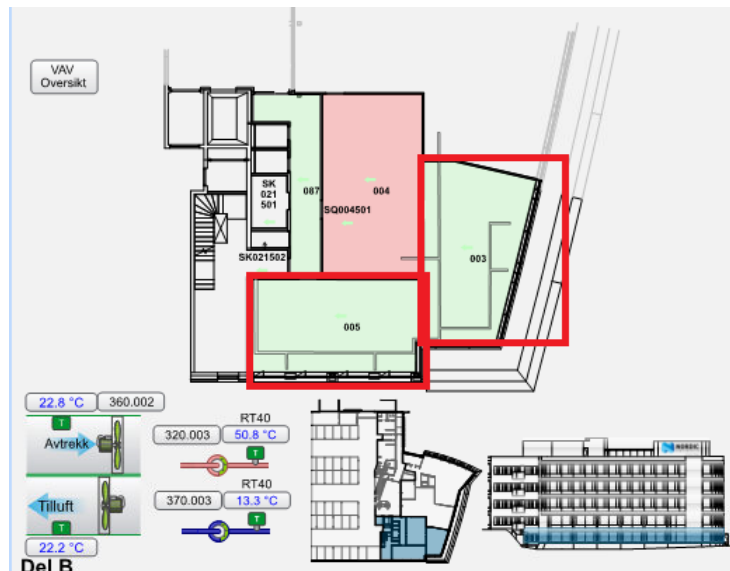
Figure 3.7: Application laboratory and support laboratory that the ventilation air flow rates are extracted from in the BOS [2]
