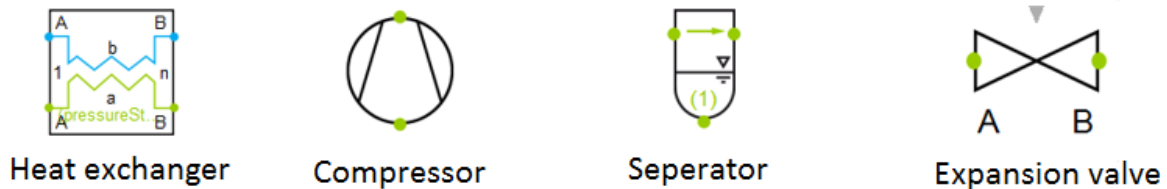
FIGURE 19: DYMOLA ICONS REPRESENTING THE MAIN HEAT PUMP COMPONENTS
