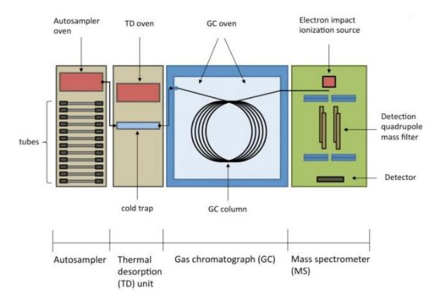
Figure 12. Autosampler connected to TD, GC and MS.
