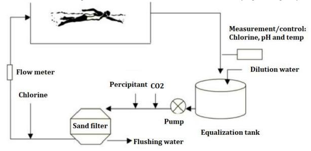
Figure 1. Normal circulation system for a swimming pool [10].
