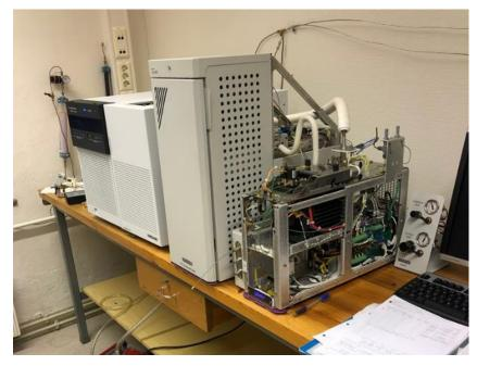
Figure 10. Station for spiking, analysing and conditioning. Gas chromatograph connected to the mass selective detector
