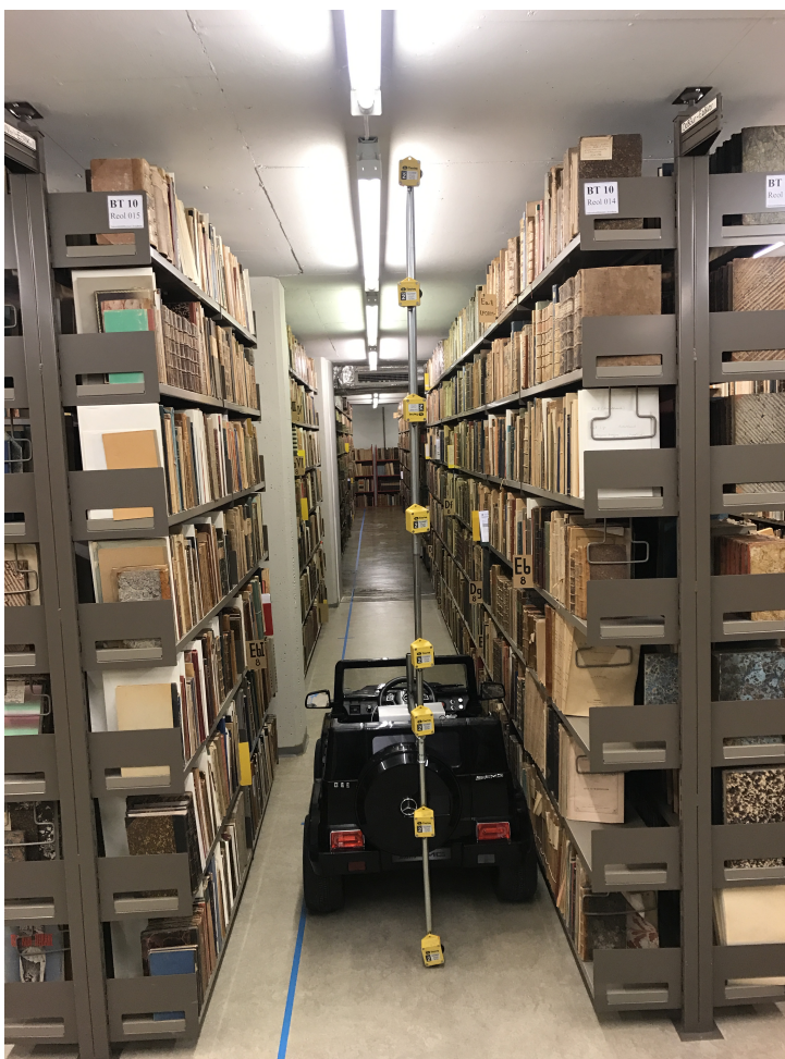
Figure 4.1: Illustration of the mobile car with the data loggers mounted on the rack
