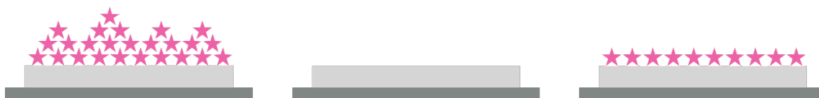
Figure 2.13: Left: Eosin Y (stars) adsorbs in multilayers onto the ZnO during the hybrid electrodeposition. Middle: The eosin Y can be removed by KOH at a pH of 10.5, leaving bare ZnO. Right: Dye molecules re-adsorb in a monolayer.
