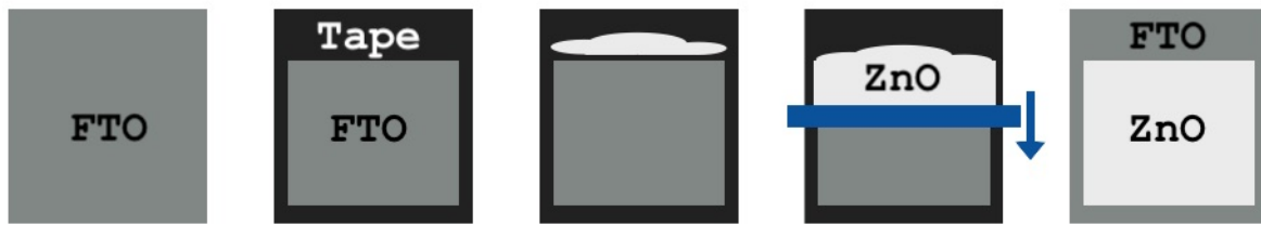
Figure 2.14: Illustration of the doctor blading process.
