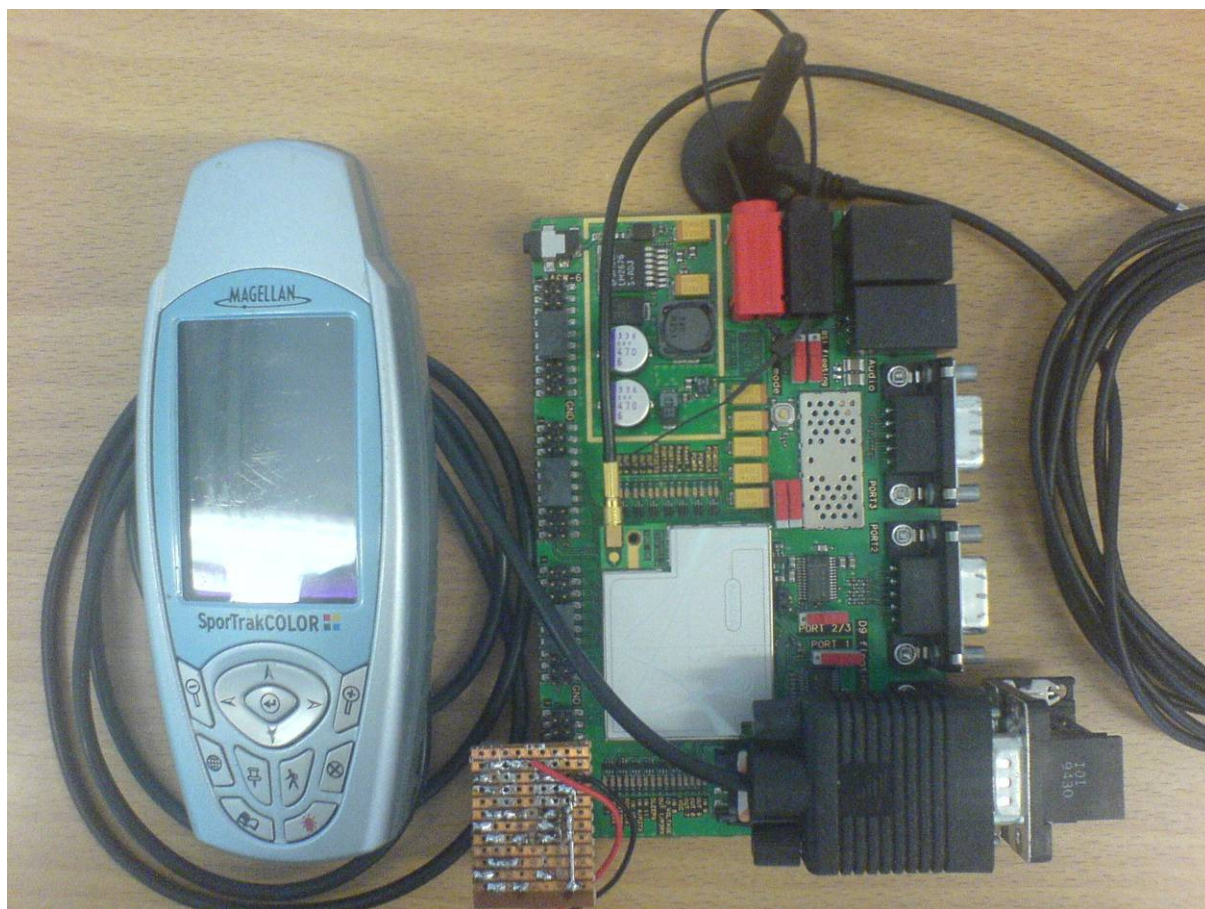
Figure 59: The Aplicom N12i module with test board and GPS
