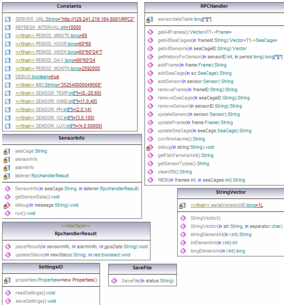
Figure 74: com.telenor.apms.fifamos.client.j2se.utils class diagram
