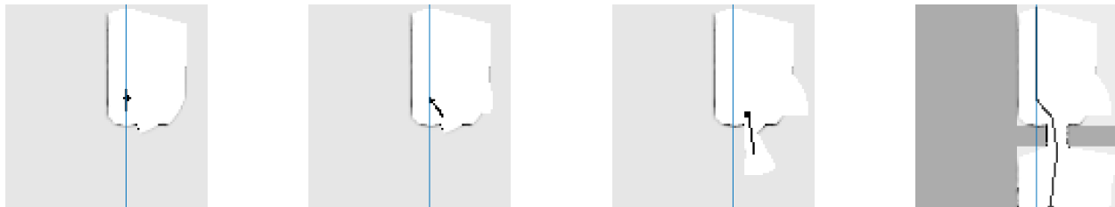
(a) The sensor cone size makes it difficult to detect if there is an opening in the wall. The drone reduces its speed and approaches slowly. (b) The drone moves towards a possible opening. (c) An opening is found and the drone flies through at full speed. (d) The final path the drone followed. The true obstacles are superimposed on the occupancy grid map.
