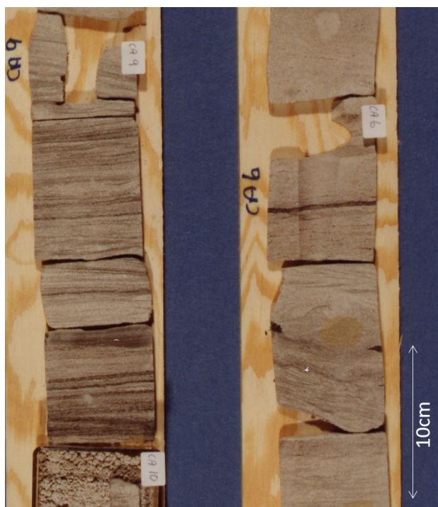
Figure 5.5: Core photo from well 6507/12-1 taken in the Åre Formation at 2520 m depth showing a light grey sandstone with abundant thin laminations of finer, darker material typical of a tidal-influenced environment (Nichols 2009)
