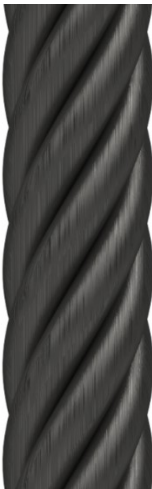
Figure 4.2 Simple twisted rope with N=6 , \theta=70^\circ , r=10mm and H=50mm
