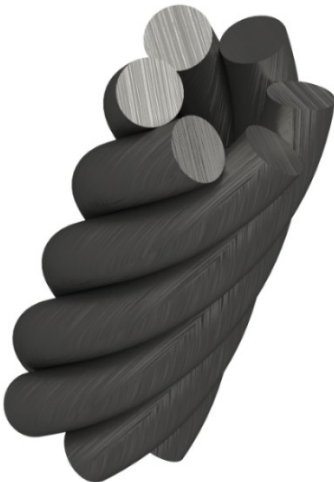
Figure 4.1 Simple twisted rope with N=6 , \theta=70^\circ , r=10mm and H=50mm
