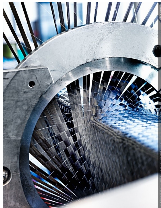
Figure 2.3 Braiding of aircraft component for Airbus (Airbus, 2017)
