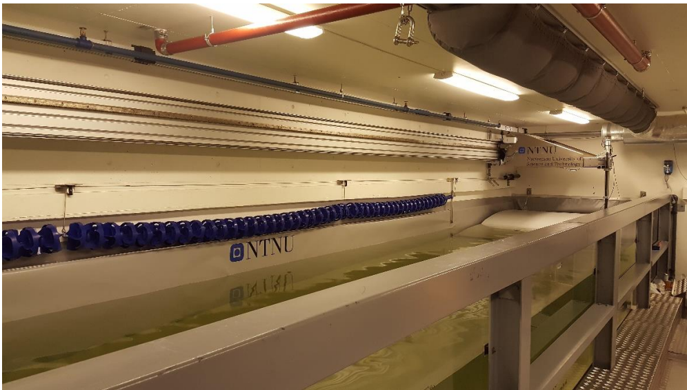
Figure 1.3 Towing tank to be used in experimental tests
