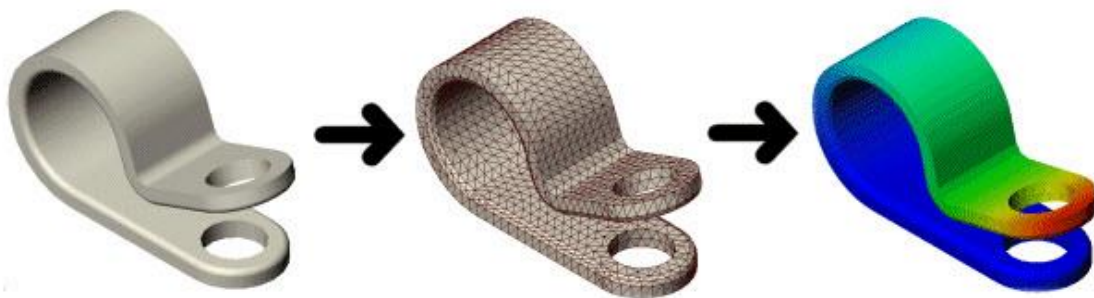
Figure 2.4 Simple FEM procedure illustration (Prokos, 2019)
