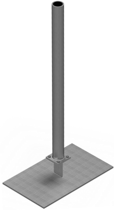
Figure 3.13 Assembly of 60 mm cylinder attached to base plate
