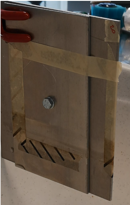
Figure 3.21: The two stainless steel plates attached with a bolt will be used to check how much biofilm can grow between the two plates.
