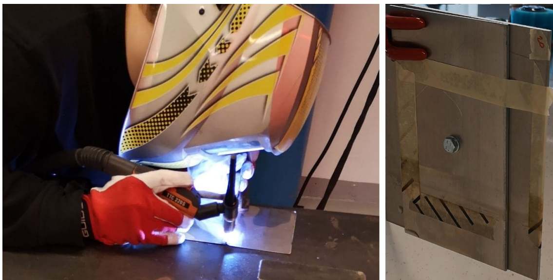
Figure 3.6: To the left: tack welding two aluminium plates together, to the right: Two stainless steel plates assembled with bolt and nut.
