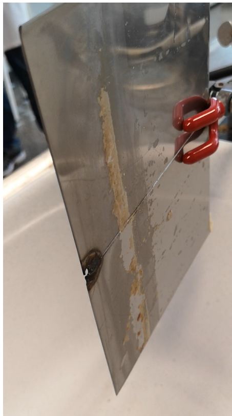
Figure 3.27: Shows a larger amount of biofilm which has lost grip of the surface of stainless steel before the cleaning has started.
