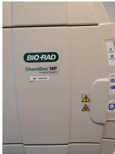
Figure 3.19: BIO RAD's ChemiDocMP designed to detect fluorescence.
