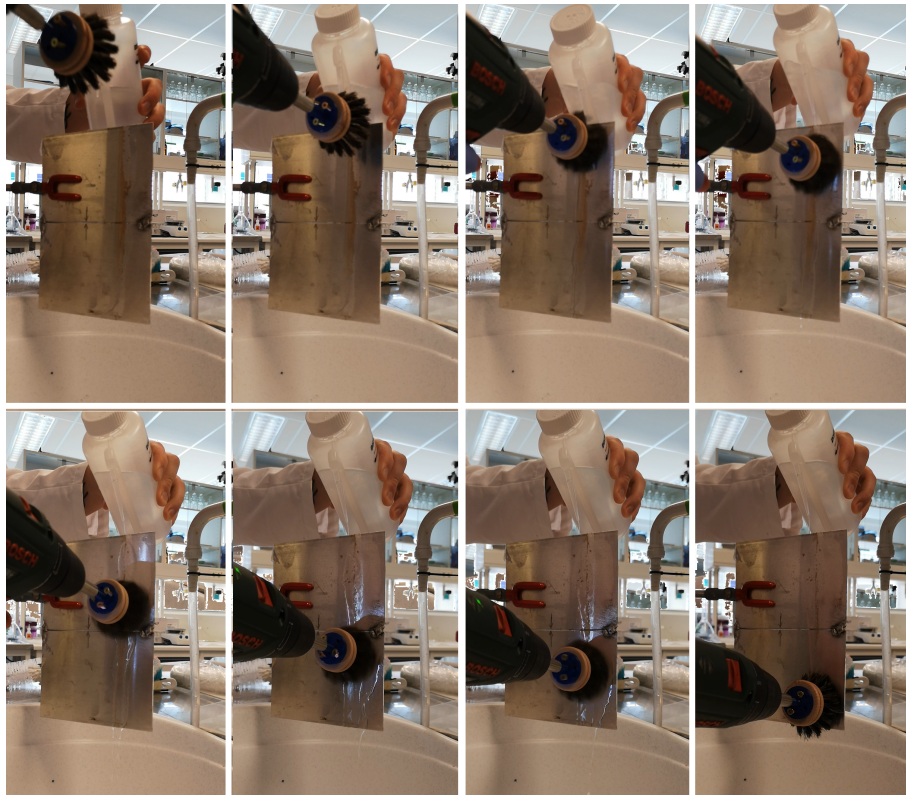
Figure 3.26: The cleaning procedure with a rotational speed close to 240 rpm.
