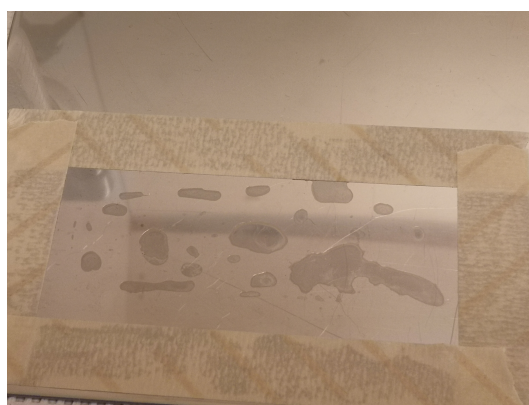
Figure 3.13: Bacteria forming biofilm onto the surface over night.
