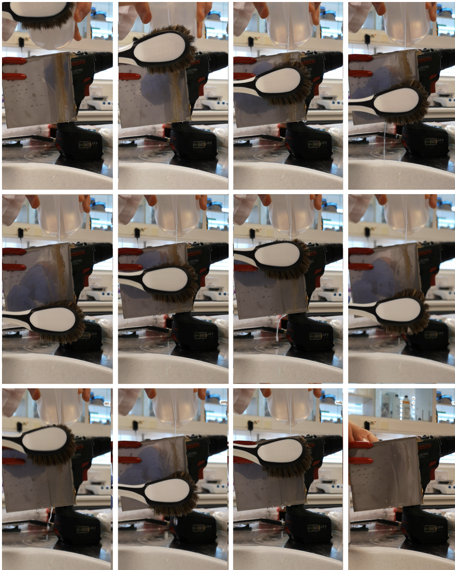
Figure 3.25: The cleaning procedure with cleaning brushes was done in a similar movement pattern as if a robot did the cleaning with slow movements back and forth.
